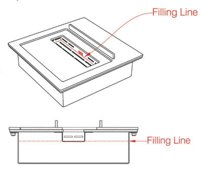
To fill the Combustion Chamber, remove it from the Main Body using the Lifting Handles and pour fuel inside the Vent Opening being careful not to spill. Fill up to the fill line as indicated in red with no more than 1,7L of fuel. After filling is done, wipe away any spilled or excess fuel before returning the Combustion Chamber to the Mount Plate opening.
