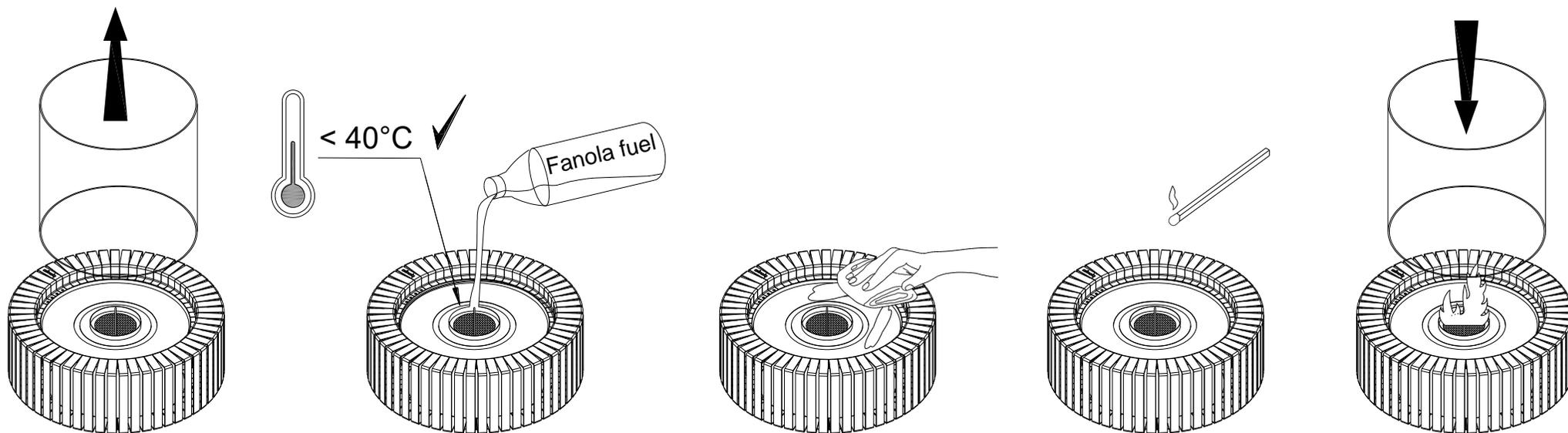
**EN** Take off the glass tube. Carefully pour fuel into the central opening of the burner (min 0,5l, max 1,5l). Warning! Fuel can only be poured into a chilled fireplace, min. 20 minutes after putting out the fire with the metal lid. Wipe away any fuel stains from the fireplace surface with a soft cloth. Light the fire with a match or lighter. Carefully place the glass tube back.
